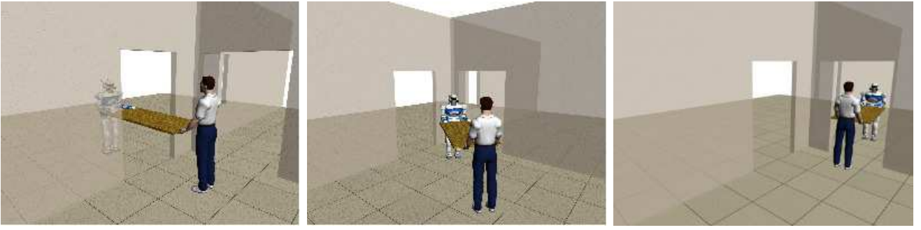
Fig. 1. Scenario of the experiment. The human-robot dyad has to carry the table through two doors that form a 90° angle. The dimensions of the table are too big to perform the task with a single bend, so that the human has to pass backward through the first door and forward through the second one. The human assumes the leadership of the task as he is walking backward through the first door, and then is guided by the robot through the second door. During this second phase, the robot is remotely controlled by a second human thanks to a joystick.
