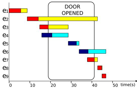
Fig. 5. Result of tasks sequencing and behavior optimization. Each task is described by two periods: the dark one is the achievement period  $[t_i^I, t_i^R]$ , the bright one is the SoT presence period  $[t_i^I, t_i^F]$ .
