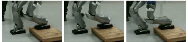
Fig. 5. The robot makes a hop after landing the left foot (the feet does not touch the ground in the middle picture and the robot is not in contact anywhere.)
