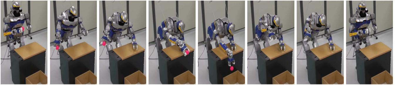
Fig. 3. The HRP-2 leans its left hand on a desk to put a ball in a box behind the desk. The motion and the position and orientation of the left hand contact are obtained by our method.
