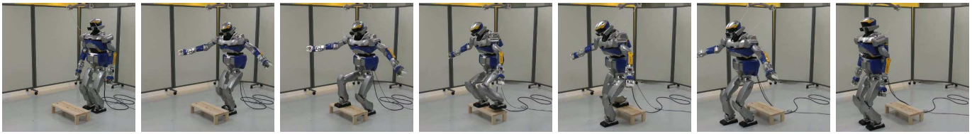
Fig. 7. The HRP-2 overcrossing a fifteen-centimeter platform: the HRP-2 takes steps the platform with one foot and over-cross it with the other.
