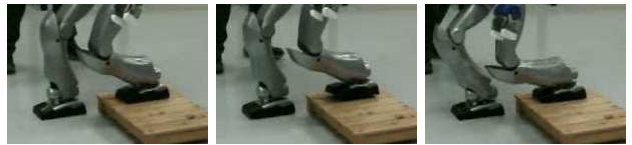
Fig. 5. The robot makes a hop after landing the left foot (the feet does not touch the ground in the middle picture and the robot is not in contact anywhere.)
