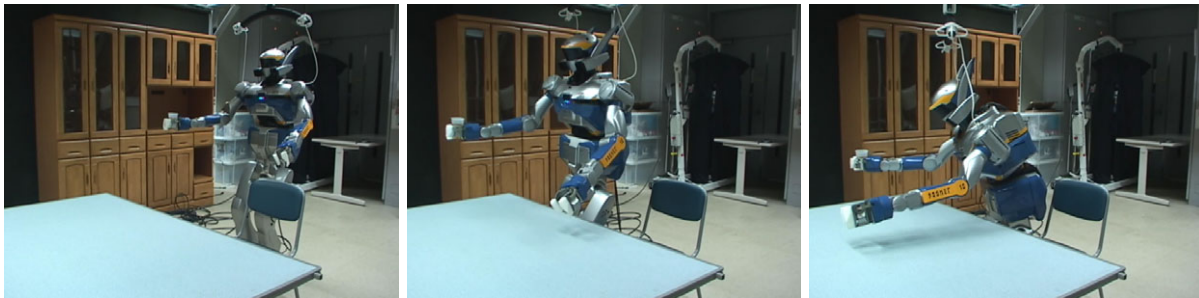
Fig. 8. The glass scenario played on HRP-2. The glass remains perfectly vertical during the whole motion.
