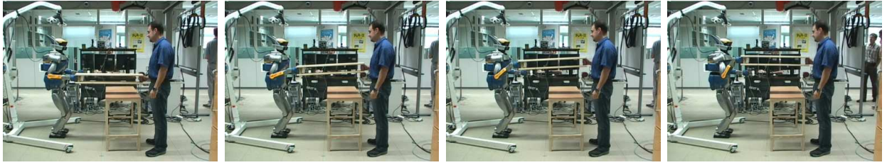
Fig. 4. Autonomous reproduction of a beam lifting task by HRP-2 jointly with a human task-partner.
