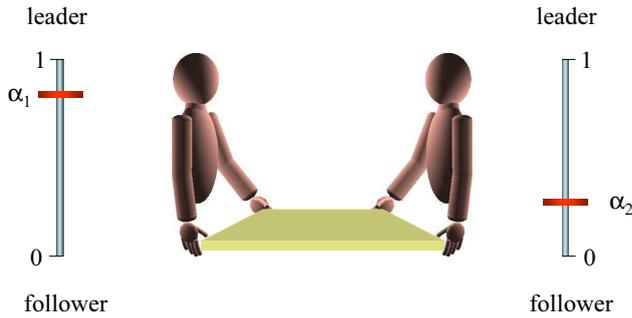
Figure 1: Illustration of one degree of freedom homotopy for each individual of the physical interaction task dyad (holding a table). Each  $\alpha_{i \in \{1,2\}}$  may evolve independently from the other and their time function results on a dynamic sliding between 0 and 1 during task execution.
