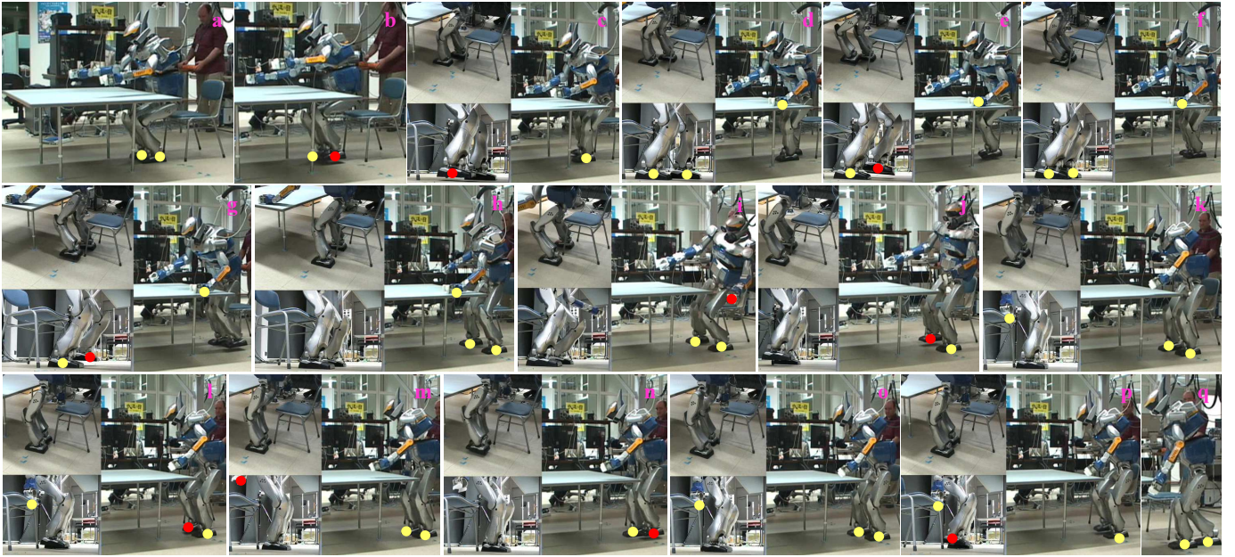
Fig. 2. Leave table experiment with HRP-2. The yellow disks highlight the HRP-2 bodies that are in contact, the red disks point on bodies that released a contact. The number of yellow disks in each picture is exactly the number of supporting contacts. The sequences are only key postures from the overall experiment described in [2]. Many transitions have not been illustrated for clarity and because of space limitation. Most pictures are having three camera views of a similar sequence: the main camera shot is shown in the main body of each picture. The left-upper small snapshots are the view of the camera put behind the chair at the left of HRP-2. The left-down small snapshots are the view of the camera put in front of the feet on the floor. (a) Initial configuration, the robot is sited on a chair in front of the table. (b) the robot lies right to ensure static balance and releases the left foot contact to replace it more on the left; after what the HRP-2 stands-up lining left and put most of its weight on the left leg (this sequence is not illustrated). (c) keeping the left foot contact, HRP-2 releases the right foot one to place it rearer, between the chair legs and ends with two contacts. (d) The planner suggests HRP-2 to take a support with its left arm on the table (3 contacts), and then performs a sequence of foot replacements illustrated by snapshots (e)(f)(g) and (h); the stances switch between 3 and 2 supporting contacts. (i) HRP-2 releases the hand contact from the table and is supported only by feet contacts. It shifts most of its weight on left one to bring the right leg near the left one (j). In sequences (k) to (p) the planner suggest taking support by the right arm on the chair allowing HRP-2 to switch between 3 and 2 contacts for shifting progressively the left and right legs and then all the robot out of the chair and table (q). Note that the hand support on the chair is made ((k) and (l)), released ((m) and (n)) and made again lefter on the chair ((o) and (p)).
