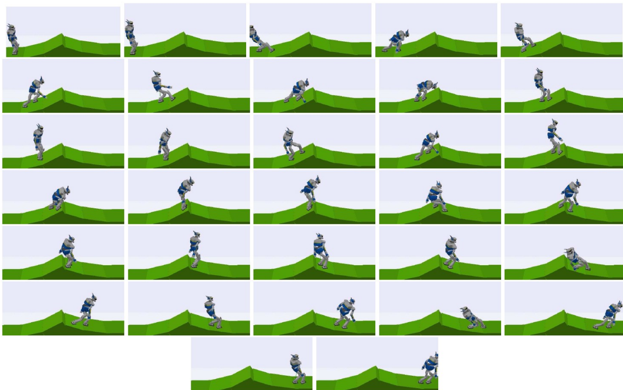
Fig.2: Locomotion over irregular terrain using Coulomb friction.
