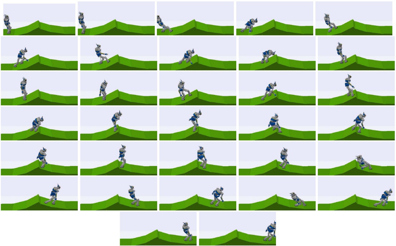
Fig.2: Locomotion over irregular terrain using Coulomb friction.
