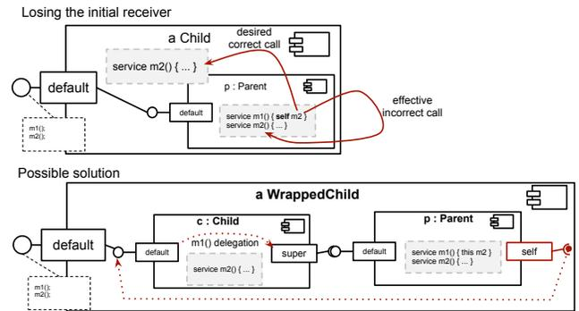
**Figure 4.** The "lost of initial receiver" problem, when composition and invocations forwarding are used. The context pseudo variable `self` does not refer to the original receiver of service invocation when delegations are used. The `m2()` service of descriptor `Child` is never called
