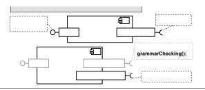
**Figure 2.** An example of an extension and specialization of required ports. Grayed parts of the figure illustrate inherited parts.
