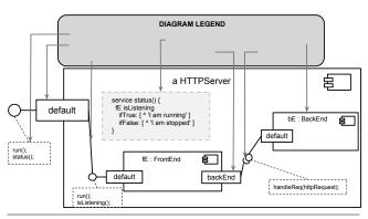
**Figure 1.** HTTPServer, the diagram shows a logical representation of an instance of the HTTPServer descriptor presented in Listing 2, after it has been created and initialized.
