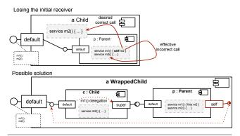
Figure 4. The "lost of initial receiver" problem, when composition and invocations forwarding are used. The context pseudo variable self does not refer to the original receiver of service invocation when delegations are used. The m2() service of descriptor Child is never called
