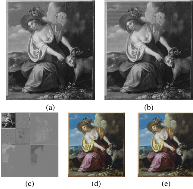
Figure 16: Application of the substitution-based approach of (R. De Queiroz and K. Braun, 2006): a) Luminance of the original color image, b) Grey-level image embedding the chrominance planes (PSNR = 28.01 dB), c) Wavelet decomposition of the grey-level image, d) Original color image, e) Rebuilt color image from the grey-level image (PSNR = 30.837 dB).
