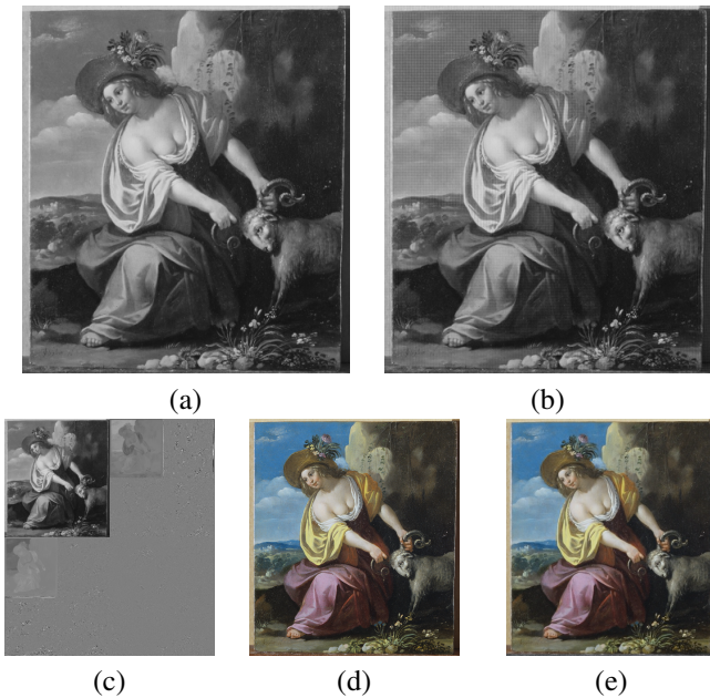
Figure 17: Application of the substitution-based approach of (Campisi et al., 2002): a) Luminance of the original color image, b) Grey-level image embedding the chrominance planes (PSNR = 33.94 dB), c) Wavelet decomposition of the grey-level image, d) Original color image, e) Rebuilt color image from the grey-level image (PSNR = 34.77 dB).
