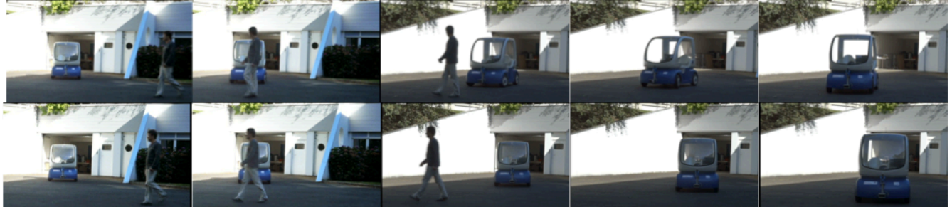
Fig. 4. First real experiment: Comparison between methods S (top) and M (bottom) as a pedestrian crosses the path in front of the robot.
