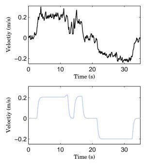
**Fig.**5 Velocities of the object on the robot's frontal axis: the admittance controller output  $\dot{\mathbf{X}}$  in black (top), robot desired velocity  $\dot{\mathbf{X}}_d$  in light blue (bottom). The role switching occurs at around t = 20s.
