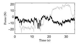
Fig.6 Force applied by the robot on the object (black) on the robot's frontal axis. The gray curve represents the damping part of the interaction force  $\mathbf{F} = -B\dot{\mathbf{X}}$ : it is the force that would be applied by the robot with a passive behavior. The role switching occurs at around t = 20s.
