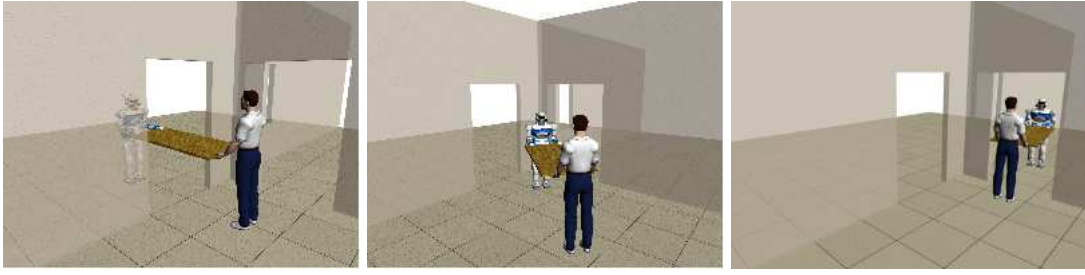
Fig.1 Scenario of the experiment. The human-robot dyad has to carry the table through two doors that form a 90° angle. The dimensions of the table are too big to perform the task with a single bend, so that the human has to pass backward through the first door and forward through the second one. The human assumes the leadership of the task as he is walking backward through the first door, and then is guided by the robot through the second door. During this second phase, the robot is remotely controlled by a second human thanks to a joystick.
