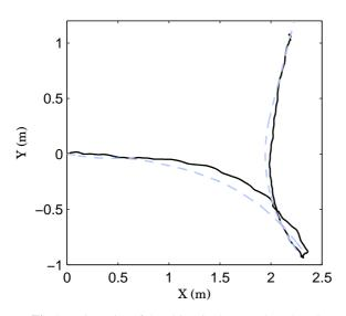
**Fig.4** Trajectories of the object in the XY plan: the admittance controller output **X** in black, follower desired trajectory  $\mathbf{X}_d$  in dotted light blue. The transportation starts at (0,0) and ends around (2,1). The role switching occurs when the object is around (2.3,-1).
