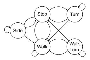
**Fig.2** Finite State Machine describing the possible primitives sequencing. It can generate sequences for both leader and follower modes. The transitions are triggered differently depending on the chosen mode.
