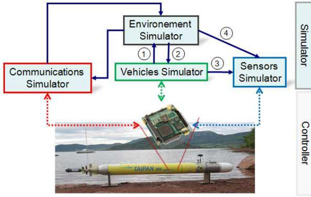
Fig. 3. Simplified architecture of *Thetis*: there is a logical sequence between 3 simulators even if there are independent processes on different computers. The cycle duration of this sequence must be largely lower than the period of the controller. The temporal decoupling is only effective (and that's enough) between the simulator and the controllers. The link between the communications simulator and the environment simulator is event-driven (when a communication between vehicles occurs).
