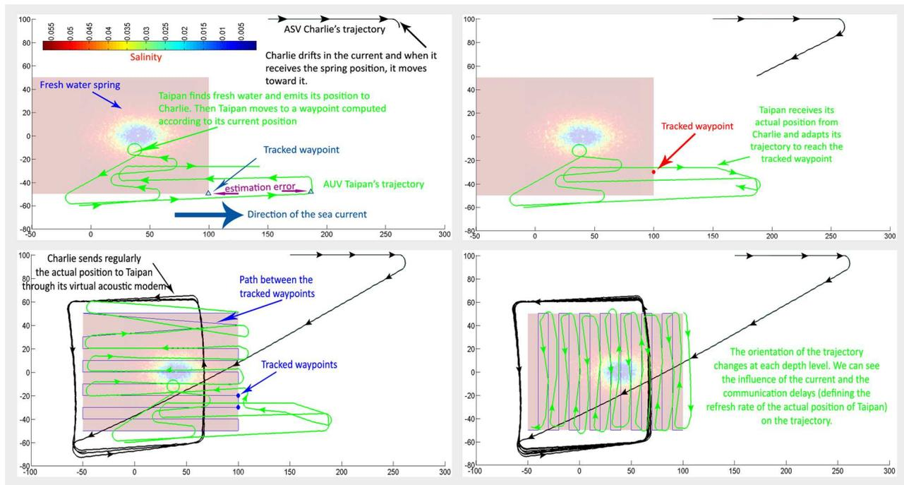
Fig. 9. *Taipan* follows the green trajectory. It is supposed to map the fresh water spring, but due to the current *Taipan* is not in the expected area. *Charlie* emits the actual position of *Taipan* through an virtual acoustic modem and *Taipan* can backtrack its actual position with an error due to the latency and the delay of propagation.
