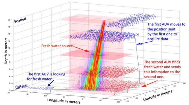
Fig. 10. The environment simulator of *Thetis* is able to represent some properties (wind, current, salinity...) of a volume using netCDF files. Two AUVs are involved here (the red and the blue trajectory). The two AUVs have to find a fresh water spring (random trajectory), and when found, the finder sends the position and the depth of the volume to be acquired to the second AUV (crenels trajectory).
