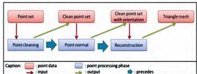
Fig. 3—Process of 3D seabed surface reconstruction
