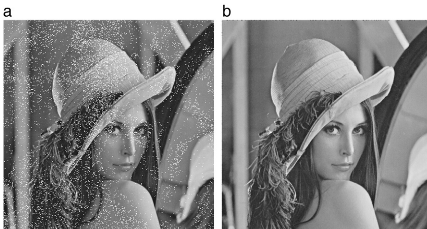
Fig. 14. a) Extracted image with blocks of two pixels, b) Reconstructed image.
