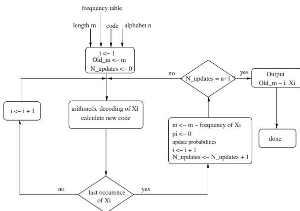
Fig. 2 Block diagram of the proposed decoding scheme.
