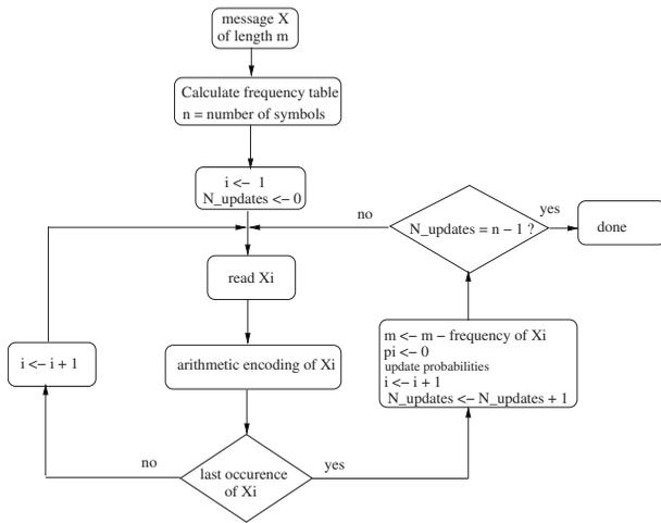
Fig. 1 Block diagram of the proposed encoding scheme.
