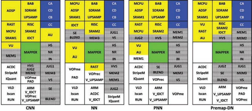
Fig. 5. Multi-task mapping in the 3x5 MPSoC, considering up to 3 tasks/PE executing simultaneously. Blue: circuit application; Yellow: MPEG4; White: VOPD; Gray: MWD. The center PE is the manager processor, which executes the *Mapper Actor*.
