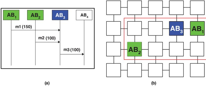
Fig. 2. (a) Application described as UML diagram, where  $m1$ ,  $m2$ , and  $m3$  represent the communication volume between tasks; (b) search space to map the  $AB_3$  task, and one possible mapping for  $AB_3$ .
