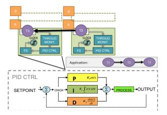
Fig. 2. Distributed PID Controllers
