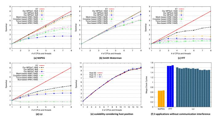
Fig. 9. Architecture scalability, for cache sizes of 4kB, 8kB and 16 kB (a)(b)(c)(d); scalability scenario regarding host position in a 4 x 4 configuration (e); cluster exploration considering MJPEG (3 threads), FFT (3 threads) and LU (15 threads), executing simultaneously (f), where each bar represents the execution time of one thread
