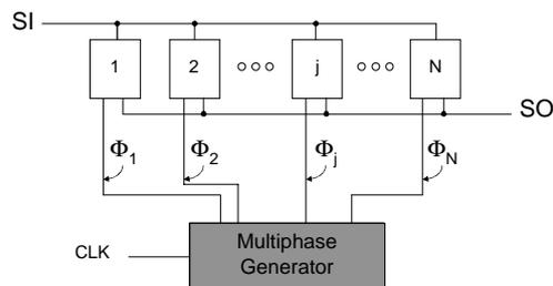
Scan architecture that uses the concept of a “token ring” to reduce shift power. SI is broadcasted to all scan cells but only one scan cell is activated at a time. An N-phase non-overlapping clocking scheme is applied with one clock for each scan cell.
