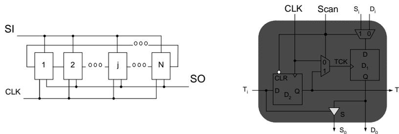
Alternative solution to avoid large area overhead of the N multiphase clock routes and inter-phase skews due to the different lengths of the N clock routes. It embeds the multiphase clock generator into each scan cell. Require the use of a new type of scan cells, called token scan cells.
