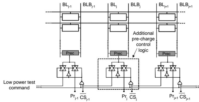
Addressing sequence is fixed to "word line after word line" and the pre-charge activity is restricted to only two columns for each clock cycle: the selected column and the following one
