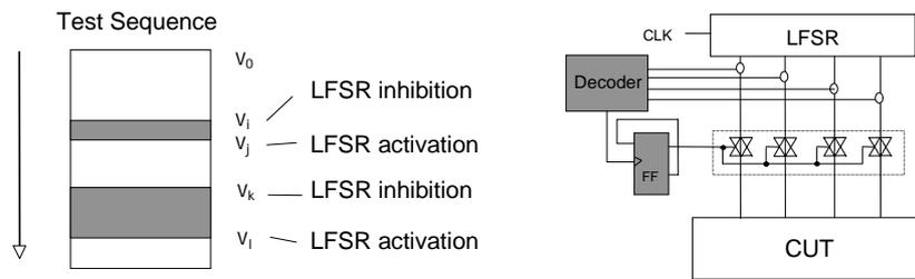
Prevent application of non-detecting (but consuming) vectors to the CUT. A decoder is used to store the first and last vectors of each sub-sequence of consecutive non-detecting vectors to be filtered.
