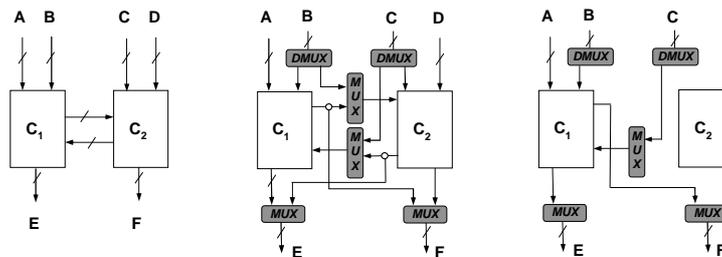
Partition the original circuit (using a graph partitioning algorithm that minimizes the cut size) into structural sub-circuits so each sub-circuit can be successively tested through different BIST sessions
