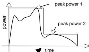
Power profile can be modified by pattern modification and/or test set reordering
