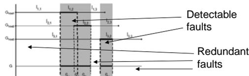
For full coverage of f, the test pattern should be applied at only two Vdd settings: Vdd2 and Vdd3 (full overlap between resistance intervals)
