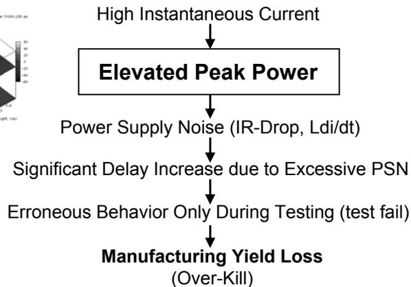
*As huge designs can be manufactured today, most power-related test issues (during scan) are due to excessive peak power*
