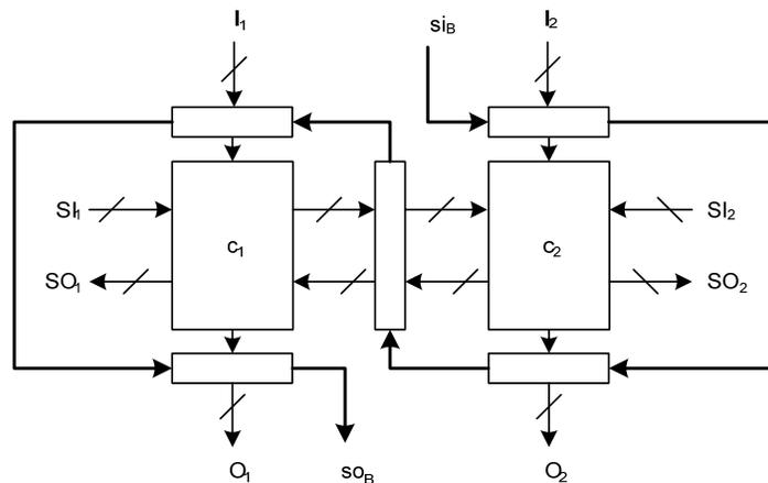
Isolating multiple cores of logic using boundary registers
