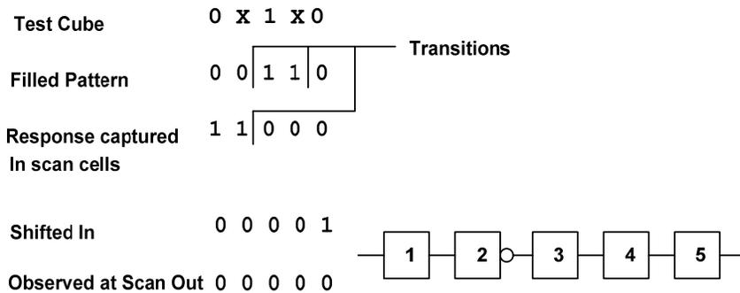
Inserting logic into scan chains to modify the transition count during shift
