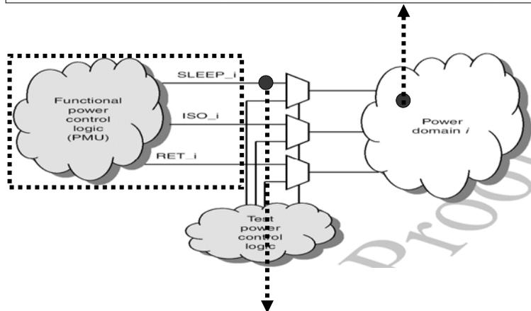
**Method-2:** *Observe at the output of the power control logic.*
