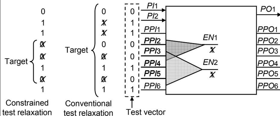
☺ Try to turn as many clock control signals into X's as possible.
