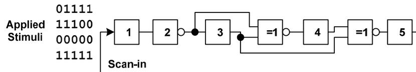
Scan segment inversion by embedding a linear function in the scan path
