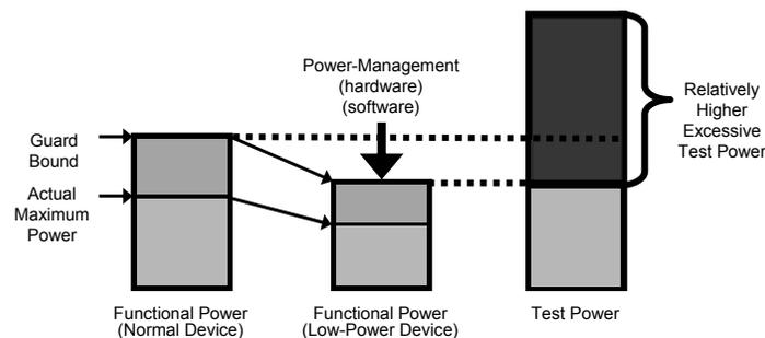
**Power during test is even more critical for low-power devices !!**
