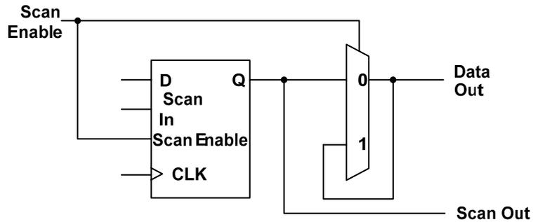
A different implementation of toggle suppression during shift using a latch at the output of the mux-D flip-flop with scan
