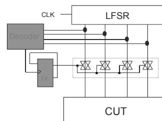
Prevent application of non-detecting (but consuming) vectors to the CUT. A decoder is used to store the first and last vectors of each sub-sequence of consecutive non-detecting vectors to be filtered.
