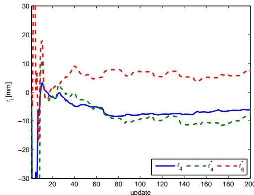
Fig. 5. Parameters of the constrained Kalman,  $\vec{r}_i^*$ , filter converges faster than the unconstrained version,  $\vec{r}_i^*$ , when the same data is given to both filters during identification.
