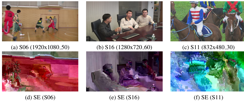
Figure 4: SE of different syntax elements for frame # 8 of several video sequences having different resolution and frame rate at QP value 18: a-c) Encoded frames, d-f) Encoded and encrypted frames.
