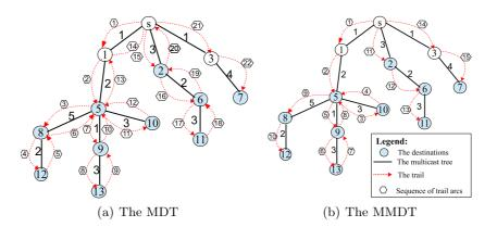
Fig. 6. Illustration of MDT and MMDT
