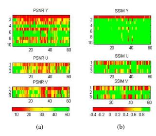
Figure 7: PSNR and SSIM of "mobile" in QCIF with QP 12 for the 60 first frames, only the 26th block encrypted.
