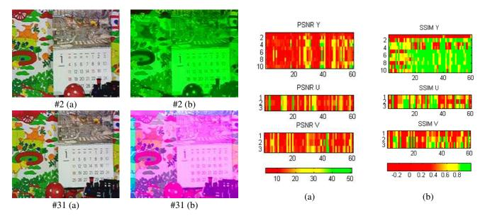
Figure 4: a) Original images of "Mobile", b) Corresponding images where only the first block is encrypted using SE [6].
