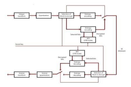
Figure 1: Block diagram of encryption and decryption process in H.264/AVC.
