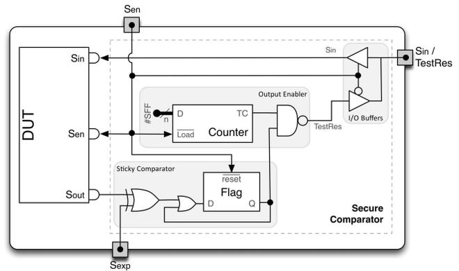
Fig. 1. Secure Comparator.
