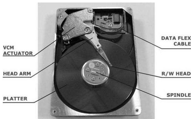
Fig. 1: View of typical components of HDD[15]
