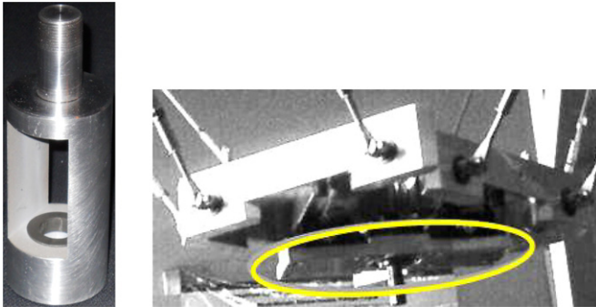
Fig. 17. Photographs of the cylindrical adaptor and the plate, which are parts of a parallel robot [28].
