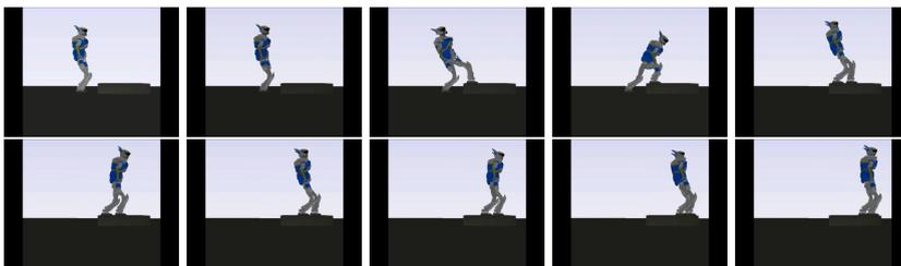
**Fig. 4.** The autonomously offline planned sequence of intermediate static configurations. The second posture removes the left foot contact from the stance by shifting all the weight on the right foot support. The third posture moves the now support-free left foot and adds it to the stance, etc.
