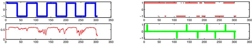
**Fig. 6.** BCI decoding performances. On the horizontal axis is step number  $t$ . From top to bottom and left to right: the command cue in thick blue, the decoded brain activities ( $P(k_t = +1|\mathbf{C}_t)$ ) in thin red, the probability 0.5 thresholded estimated classified label (ie.  $P(k_t = +1|\mathbf{C}_t) \geq 0.5$  or  $< 0.5$ ) in thick red point marker, the command  $c_t$  sent to the robot (based on the threshold  $P_{\text{thres}} = 0.6$ ) in thick green.
