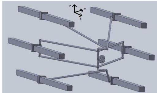
Figure 2. Simplified CAD drawing of the mechanism for clarification purpose only. The rotation of the platform is greater than  $90^\circ$ . The x, y and z directions of the base frame are shown in the figure.
