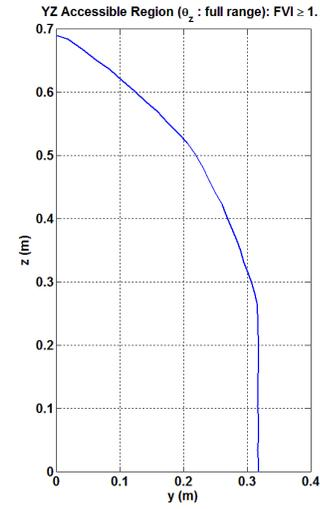
Figure 6. Boundary of the accessible yz region with full orientation capability (between  $-90^\circ$  and  $+90^\circ$ ). It has been shown on the quarter of the workspace due to symmetry with respect to the y-axis and z-axis.
