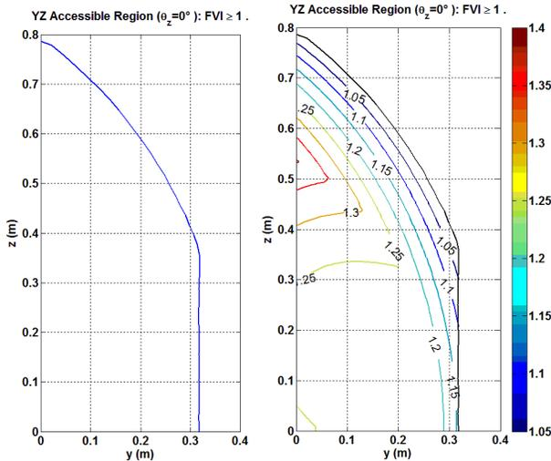
Figure 5. On the left we show the boundary of yz region accessible with null orientation. On the right we show the contour plot showing the variation of the FVI index as function of the position  $(y, z)$  in the case of null orientation. These have been shown on the quarter of the workspace due to symmetry with respect to the y-axis and z-axis.
