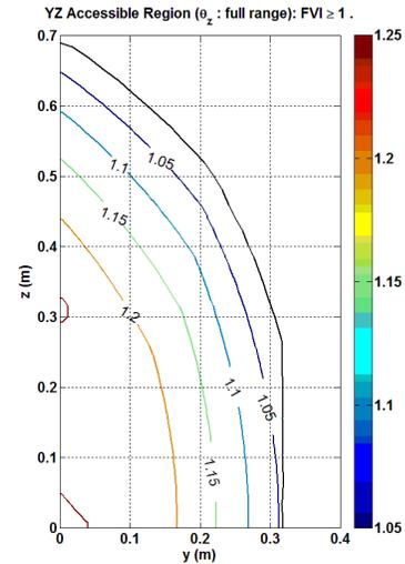
Figure 7. Contour plot showing the variation of the index FVI as function of the position  $(y, z)$  and for full orientation capacity (the value shown at each position is the worst value (smallest) of the index among the different angles tested between  $-90^\circ$  and  $90^\circ$ ). It has been shown on the quarter of the workspace due to symmetry with respect to the y-axis and z-axis.
