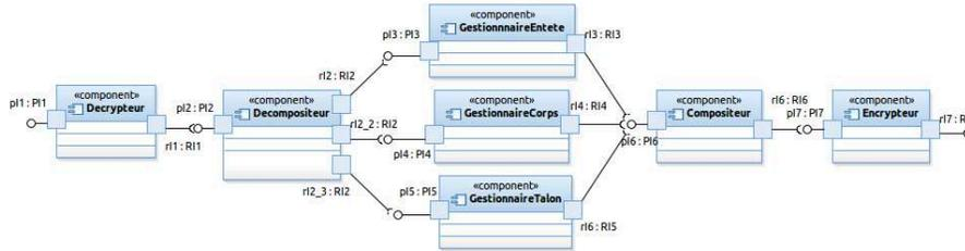
Figure 2.8. Illustration du style d'architecture Pipe and Filter
