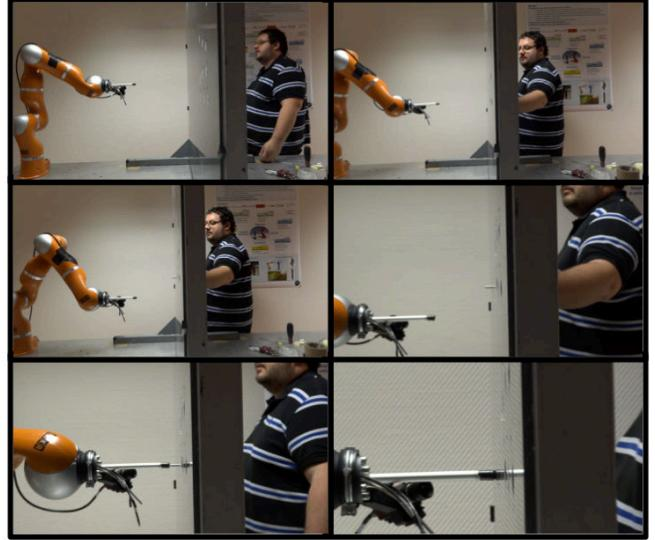
Fig. 4. Snapshots of the experiment of collaborative screwing.
