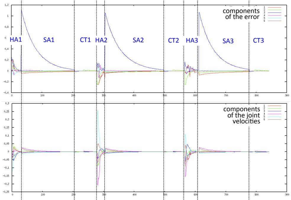
Fig. 3. The six components of the error  $\mathbf{e} = \mathbf{s} - \mathbf{s}^*$  (top) and the seven components of the articular joint velocities  $\dot{\mathbf{q}}$  (bottom) during the experiment. The error components  $e_1$ ,  $e_2$ , and  $e_3$  for HA and CT are expressed in meters,  $e_3$  for SA is in log meters, and  $e_4$ ,  $e_5$  and  $e_6$  are in radians. The articular joint velocities are all expressed in rad/s.
