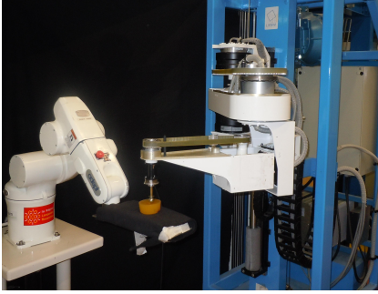
Figure 11: Experimental platform for motion compensation: The D2M2 robot is running the force control and the Viper Robot performs the disturbance motion. The force control is used to keep the contact force constant even in the presence of disturbances.
