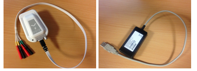
Fig. 2. Wireless stimulator (Left) with its control unit (Right)
