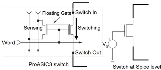
Fig. 9. ProASIC3 actual switch (left) and the simplified switch modeled in SPICE by a NMOS pass-transistor (right).
