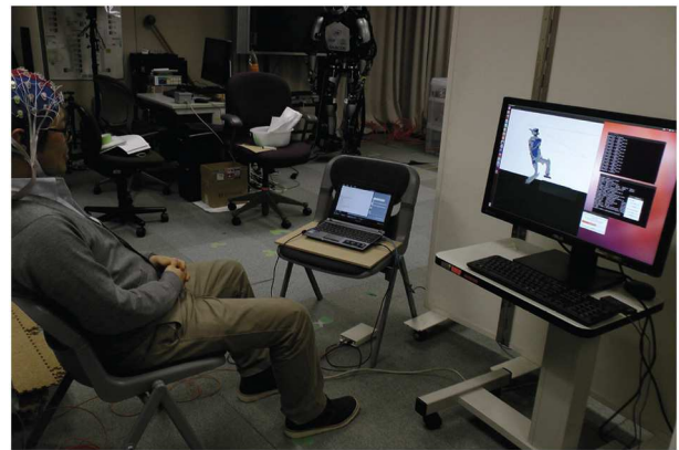
FIGURE 3 | Experiment setup. The user is wearing an EEG cap. The laptop on his left side is used for decoding the motor imagery task signal, the computer on his right runs the real-time physics simulation allowing him to control the position of the moving foot through the visual feedback he gets from the simulator window.
