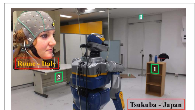
FIGURE 1 | Participants located in Rome (Italy) controlled an HRP-2 humanoid robot located in Tsukuba (Japan) by a SSVEPs-BCI system.
