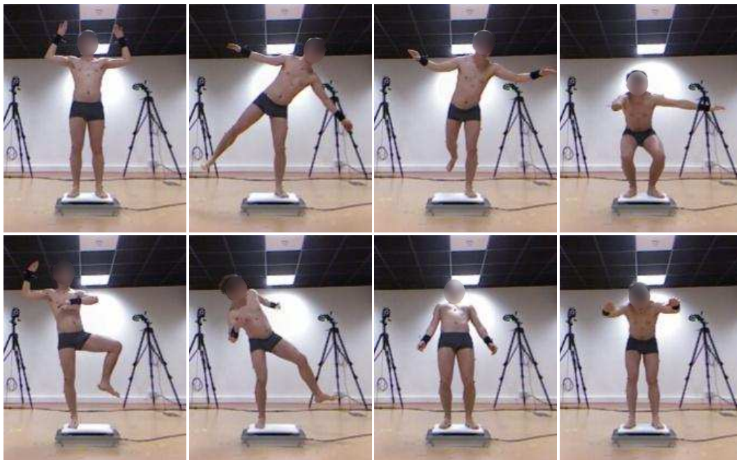
Figure 2. Synchronous recording of Vicon-AMTI-OR6 (AMTI6 by Advanced Mechanical Technology, Inc.) and Kinect-Wii balance board (WBB by Nintendo® Company) measurements. Measuring the same postures with both sets of sensors allows the comparison of SESC-based CoM estimations. Please refer to the Supplementary Material for complete list of postures.
