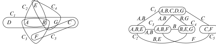
Fig. 1: Hypergraph of a CSP example. Fig. 2: Dual graph of CSP in Figure 1.
