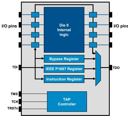
Figure 2. IEEE P1687 hardware architecture
