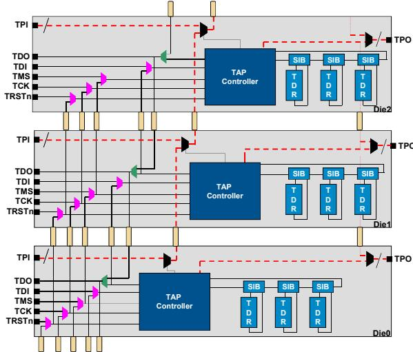
Figure 5. IEEE P1687 based 3D DFT architecture
