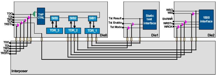
Figure 6. 3D DFT Architecture of a 3D circuit on passive interposer
