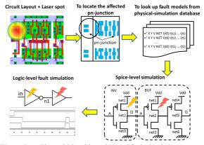
Figure 5. The multi-level laser-induced fault simulation process
