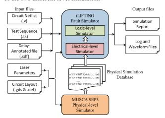
Figure 4. From physical-level to logic-level laser-induced faults simulation architecture
