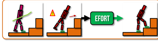
Fig. 5 Contacts are generated when the configuration is not balanced.
