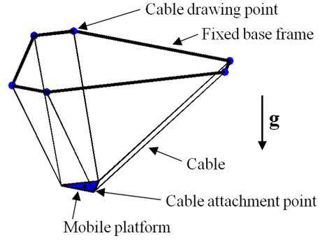
Fig. 1. Sketch of a cable-suspended parallel robot.
