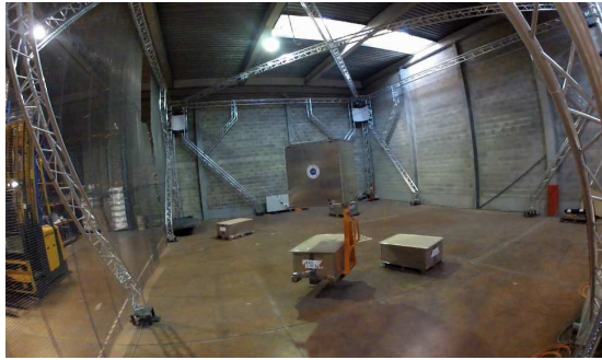
Fig. 11. The large cable-suspended parallel robot of the project CoGiRo [35]—Robot overall dimensions 15 m x 11 m x 6 m (L x l x h).
