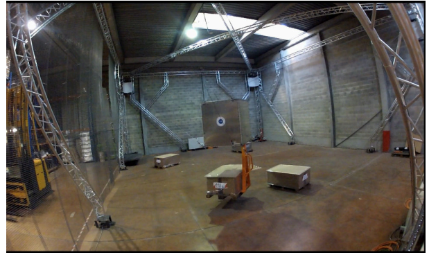
Fig. 2: LIRMM/Tecnalia CoGiRo prototype of global dimensions 15m \times 11m \times 6m ( l \times w \times h )
