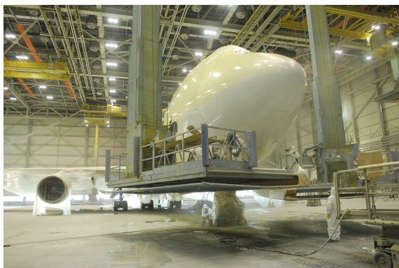
Fig. 1: Carrying workers by gantry nacelles in an airplane maintenance workshop
